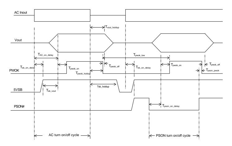
Figure 3: Turn On/Off Timing
